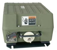
The RF-382A Series couplers efficiently and automatically match the output of 125 to 400 watt transceivers to a wide variety of whip, dipole, and long-wire antennas over the frequency range of 1.6 to 30 MHz. Tuning time from memory is less than 200 milliseconds.
