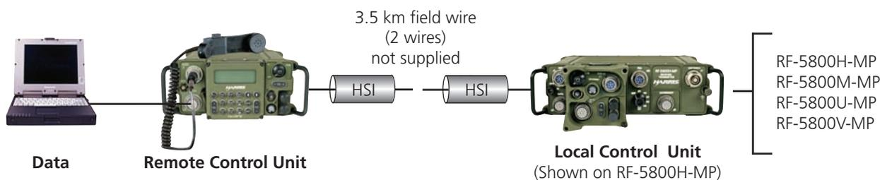
High Performance Waveform (HPW) capability can be added to the RF-5800R-RC111 Remote Control System with High Speed Interface (HSI) by adding the HPW Upgrade Kit. Order model number RF-5800R-UK200 Upgrade Kit.
