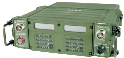
The Tactical Retransmission Unit (TRU) is a small, lightweight extension to the FALCON II® family of tactical radios that allows encrypted voice or data transmission range to be extended in a repeater or rebroadcast configuration.
