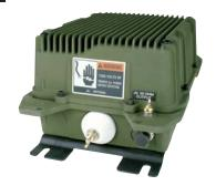
The RF-5382H coupler automatically matches the output of FALCON® II Series HF transceivers to a wide variety of whip, dipole, and long-wire antennas over the frequency range of 1.6 to 30 MHz. The antenna coupler tuning time from memory is less than 150 milliseconds and it operates at power levels from 20 to 150 watts.
