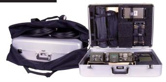
The SATCOM Radio Suitcase System is designed to transport and rapidly deploy the AN/PRC-117F(C) manpack radio for use with with SATCOM or LOS networks.
